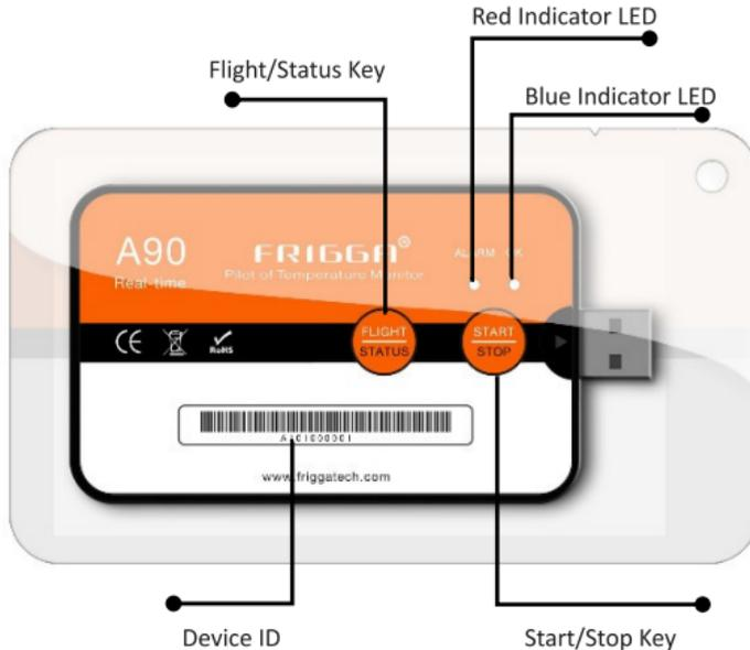
Note: The AC code (Activation code) is in the back of device.
